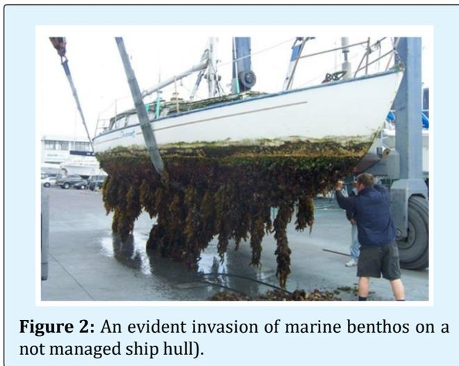
**Figure 2:** An evident invasion of marine benthos on a not managed ship hull).
