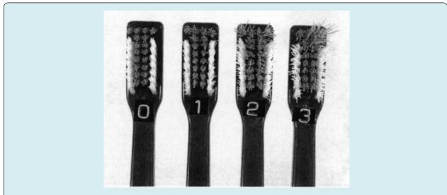
**Figure 4:** Visual comparison of the subjective wear rating scale5: 0 = None, 1 = Low, 2 = medium, 3 = High [5].
